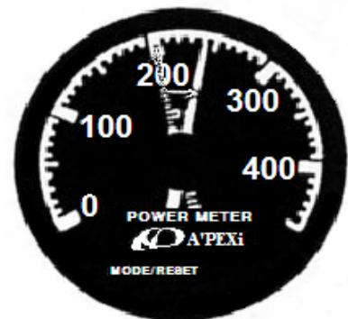
For example, if the chassis dynamometer display 240 PS and the meter only show 200 PS, turn the calibration volume towards the + side while the meter is in peak hold mode until the needle hits 240 PS. (figure on right)
